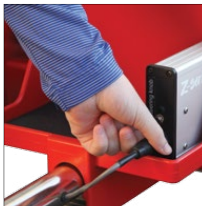
Attaching electrical connection to Z-box.
