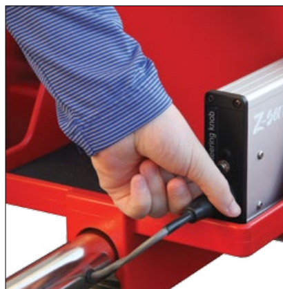
Attaching electrical connection to Z-box.
